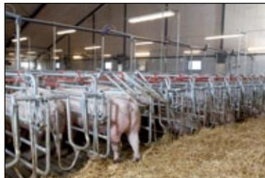
*"The free access stall has the absolute best working conditions. The sows quickly learn how to operate the stall, they have a free vision of the trough through the grille of the front gate and the front ends of the partitions are closed, providing the necessary peace when they are eating and resting"*
